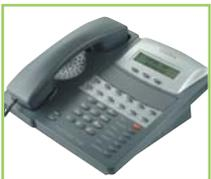
Its onboard SIP support for peer-to-peer calling makes the Edge 300 a powerful endpoint for busy professionals. Edge 300 features include an intuitive, menu-driven LCD user interface, speakerphone, headset port and built-in 2-port Ethernet switch for PC and network connectivity. The Edge 300 is available with 12 or 24 programmable buttons illuminated with tri-color LEDs.
